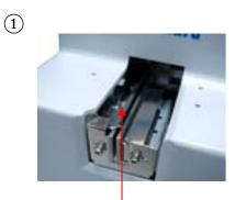
Loosen the set screw on the rail
