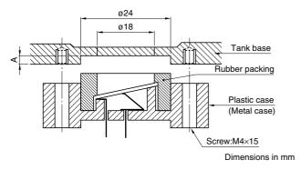
The transducer can beak off if the A dimension depth is shallow. TDK recommends a 2mm A-dimension depth and a screw tightening torque of 0.6N • m.
